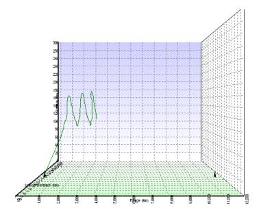
It looks like ducting in the nighttime electron density valley is a possibility for this QSO on 630-Meters. It should be noted that now the ordinary wave has excessive absorption, and the extraordinary wave is the likely candidate. I believe this is due to 630-Meters being <u>below</u> the electron gyro-frequency (the frequency at which electrons spiral around magnetic field lines).
