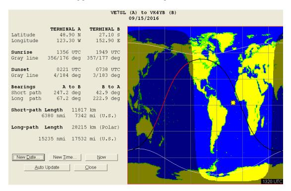
The red line is the short path between VE7SL and VK4YB. As expected, this QSO took place near sunrise on the eastern end of the path. On our low bands (especially 160-Meters), this condition can produce a sunrise enhancement in signal strength. It is likely to happen on 630-Meters, too.
