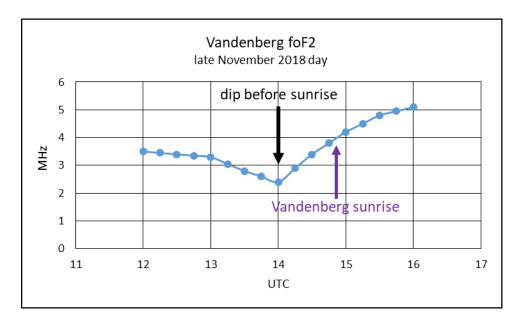
Two observations are obvious. One, the high-angle MUF [note 1] for several hours before sunrise is at or below 3.5 MHz – communication could be tough with close-in stations on 80m. Two, there is a pronounced dip in foF2 before sunrise. What's causing this dip?
