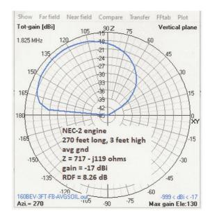
The F/B ratio (front-to-back) looks good and the RDF is good. This isn't bad for a short Beverage (if it's true!). But the back half of the elevation pattern looks kind of funny.
