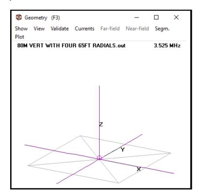
I moved the entire system from a height of 40 feet over average ground using the 'real ground' (Sommerfeld-Norton) option to a height of 0.1 feet (1.2 inches). At each height the length of the vertical portion was varied to maintain resonance near 3.525 MHz. The results were as follows.
