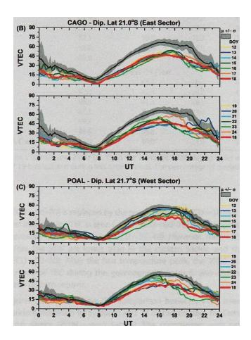
The black line with the gray shading around it is an average non-stratwarm days, with the gray shading indicating the plus/minus 1 standard deviation limit. The different colors are the different days, with the DOY legend on the right next to the color legend.
