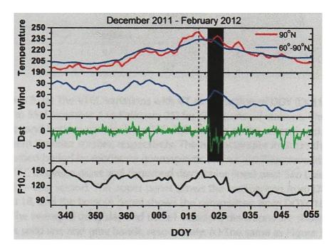
The authors state that the warming began on December 24, 2011 (DOY = day of year = 359) and lasted until February 3, 2012 (DOY = 34). Also plotted are the stratospheric zonal wind, the Dst (an indication of how disturbed the Earth's magnetic field is, with negative values being more disturbed) and the 10.7 cm solar flux. The black rectangle highlights the days when the Earth's magnetic field was most disturbed.
