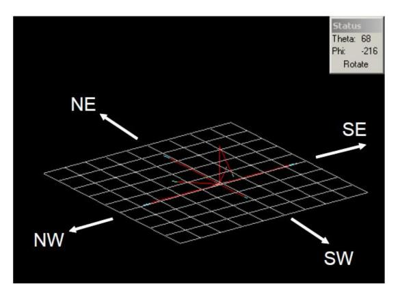
As mentioned earlier, tuning the 80m portion was easy using a small Miniductor to resonate it to 3550 KHz. The 160m portion was tuned to 1830 KHz by varying the length of the slanted wire. The modeled SWR at the antenna was as follows, and actual SWR measurements were extremely close to the modeled values.
