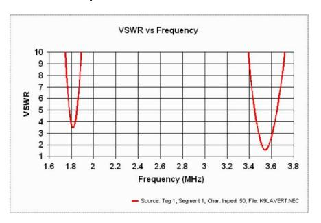
The impedance on 160m was around 15 ohms. After about 200 feet of RG-8 coax, the SWR was around 2.5:1 – my Commander HF-1250 amplifier had no problem loading
