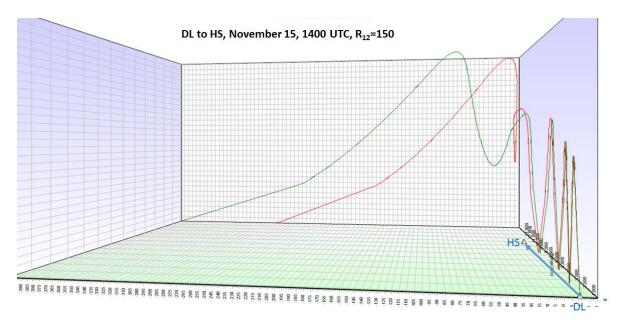
The red trace is the ordinary wave, and the green trace is the extraordinary wave. The blue arrow line is the great circle path from DL to HS (80.2 degrees). The horizontal axis is the lateral distance (in km) off the great circle path. The rays are at an elevation angle of 10 degrees.
