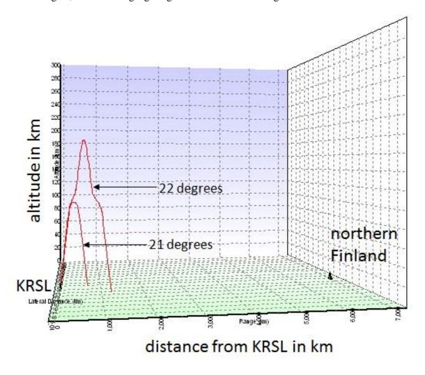
What we see are two ray traces – one at a 21 degree elevation angle out of KRSL and one at a 22 degree elevation angle out of KRSL [note 3]. The 21 degree trace gives an E hop (maximum altitude of about 90 km), whereas the 22 degree trace gives an F hop (maximum altitude of about 185 km).
