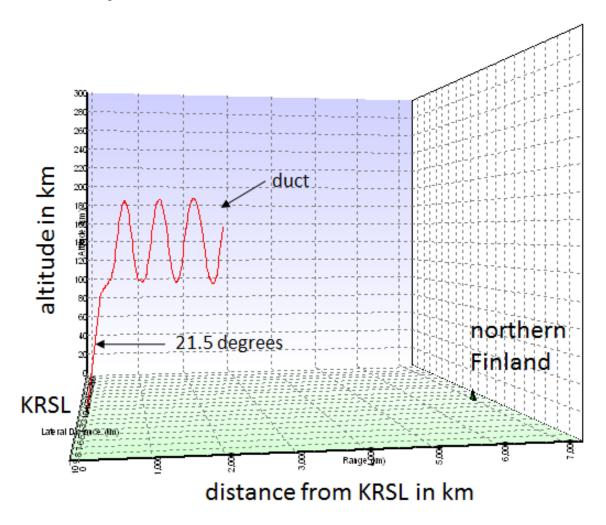
Indeed, Proplab shows a duct mode. What a duct offers is the absence of transits through the absorbing region (lower E region during the night) and the absence of ground reflections – both of which add loss to reduce the signal strength.
