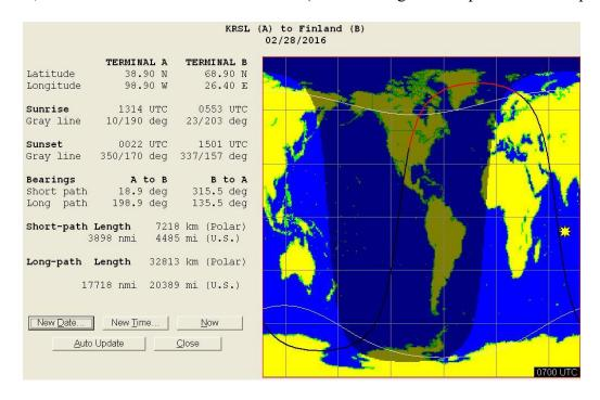
The important observation to make is that northern Finland is around sunrise [note 1]. This condition of sunrise on the eastern end of a path on our Amateur Radio low bands has been known to provide a significant enhancement in signal strength, and I'm assuming it's important on 990 KHz, too. The cause of a sunrise enhancement is believed to be due to the signal being dumped out of a duct [note 2] as a result of the tilted ionosphere at sunrise. Thus we'll look for evidence to support a duct.
