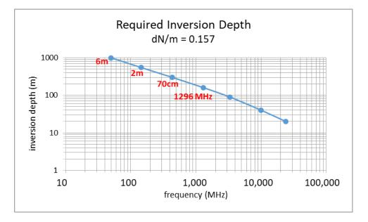
The original figure only went down to 432 MHz (70 cm), so I extrapolated the data down to 50 MHz (6 meters).
