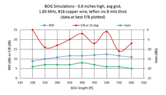
Again, what stands out is the cyclic nature of the F/B ratio. Just like the normal Beverage, there are preferential lengths of BOGs for optimum F/B performance. The first F/B peak is at a length shorter than a normal Beverage due to the velocity of propagation on the wire decreasing as it is brought closer to ground.
