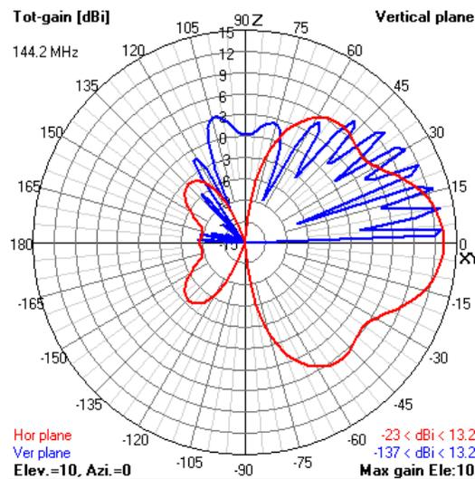
The gain on 2m is 13.2 dBi, which translates to about 6 dB over a 6m dipole at the same height. Note that the active region of this LPDA at 144.2 MHz (based on the currents) is for all intents and purposes element 13 through element 20 (the shortest element).
