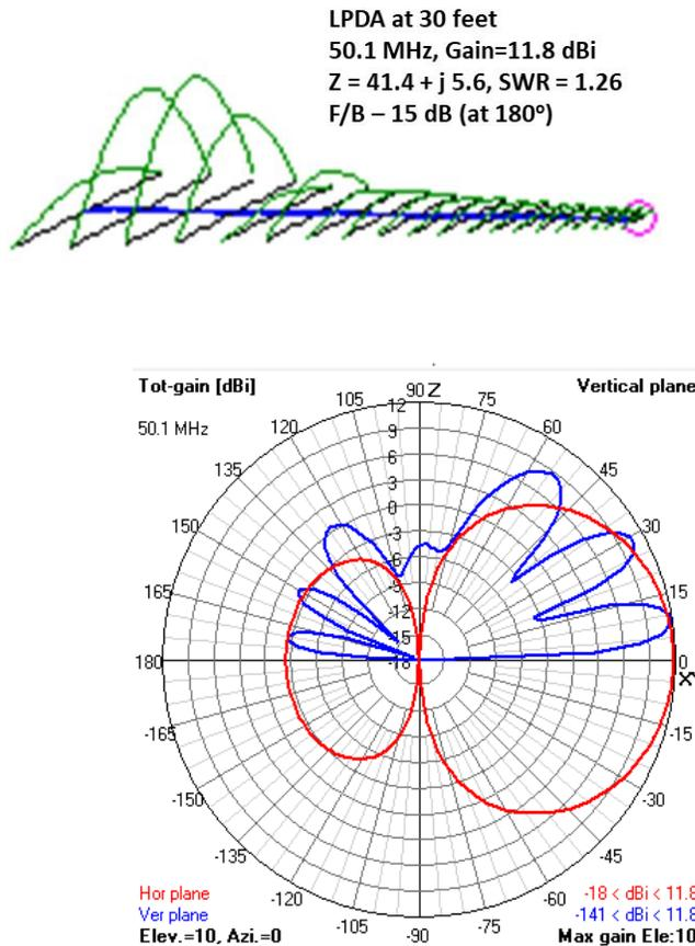
The gain on 6m is 11.8 dBi, which translates to about 5 dB over a 6m dipole at the same height. Note that the active region of this LPDA at 50.1 MHz (based on the currents) is for all intents and purposes element 1 (the longest element) through element 7. Now let's look at this design at 144.2 MHz.
