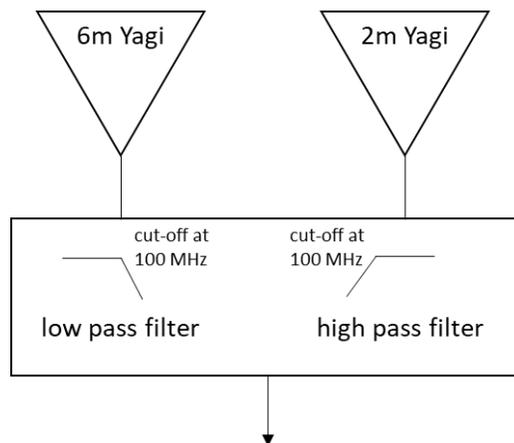
In addition to the basic low-pass and high-pass functions, each filter must present a high impedance to the other frequency [[note 3](#)].
